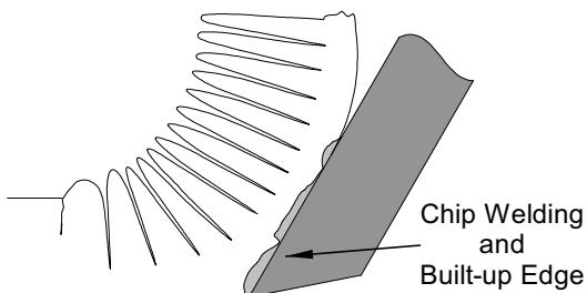
Built-up edge occurs when the SFM is too low to generate enough heat to keep chips from pressure welding to the Insert. This results in poor finish and edge chipping. Increased SFM, positive rake geometry and coated Inserts reduce chip welding. Use grades 110 or 310 to resist chipping when the SFM can not be sufficiently increased.
