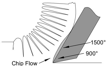
Under optimum cutting conditions, the underside of the chips soften to become almost fluid as they pass across the Insert. This helps chips flow easily out of the cut. The flow zone behind the cutting edge is where the highest heat and pressure develops. Cratering can also occur in this area.
