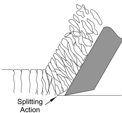
Cast Iron, Hard Brass and other materials that produce powdery chips
